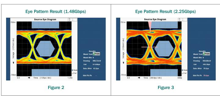
Figure 2 and Figure 3 respectively shows the passing eye pattern result using Semtech's RClamp0524P.
