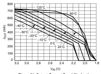
Figure 21. Output Current Capability for the 1.8 V Version
