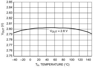
Figure 7. Output Voltage vs. Temperature 2.8 V Version
