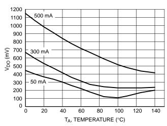
Figure 14. Dropout Voltage vs. Temperature 1.5 V Version
