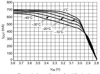
Figure 19. Output Current Capability for the 2.8 V Version
