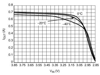
Figure 18. Output Current Capability for the 2.85 V Version
