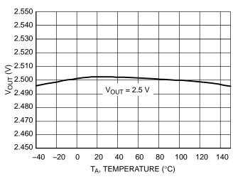
Figure 8. Output Voltage vs. Temperature 2.5 V Version
