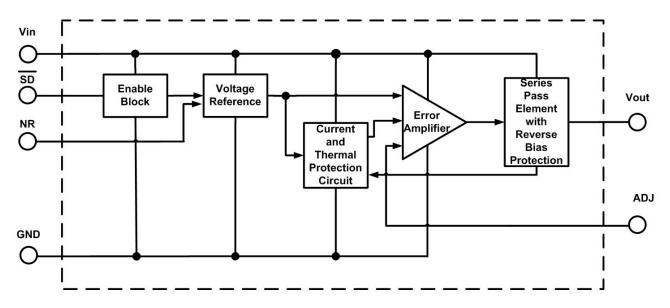
Figure 4. Block Diagram, Adjustable Output Version
