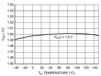
Figure 10. Output Voltage vs. Temperature 1.5 V Version
