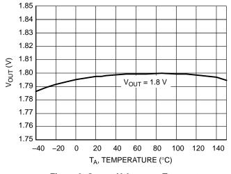
Figure 9. Output Voltage vs. Temperature 1.8 V Version
