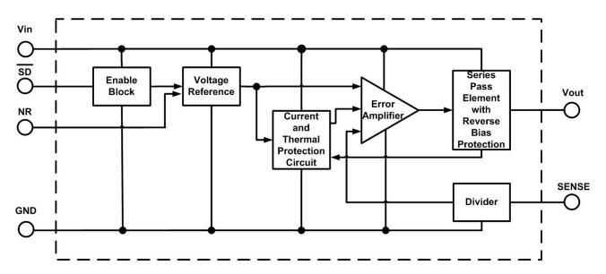
Figure 3. Block Diagram, Fixed Output Version
