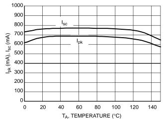
Figure 15. Peak and Short Current vs. Temperature
