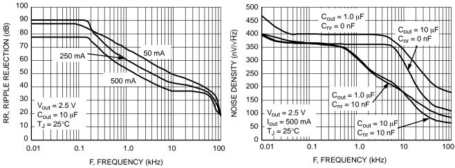
Figure 23. Ripple Rejection vs. Frequency
