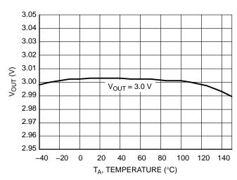
Figure 6. Output Voltage vs. Temperature 3.0 V Version
