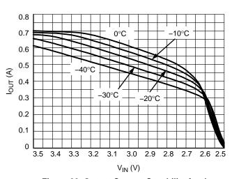
Figure 20. Output Current Capability for the 2.5 V Version
