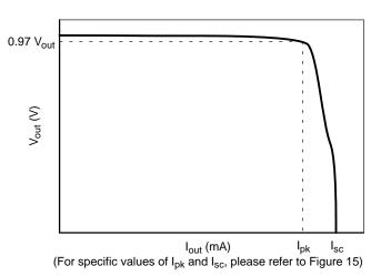
Figure 16. Output Voltage vs. Output Current
