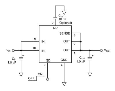
Figure 1. Typical Fixed Version Application Schematic
