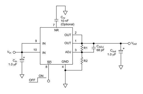
Figure 2. Typical Adjustable Version Application Schematic
