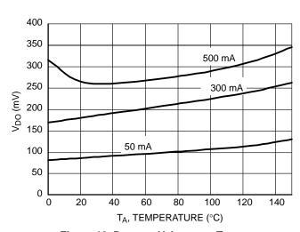
Figure 12. Dropout Voltage vs. Temperature 2.5 V Version
