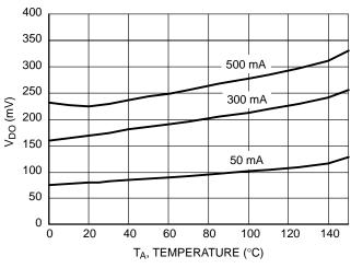
Figure 11. Dropout Voltage vs. Temperature 2.8 V Version
