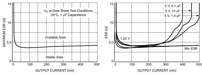
Figure 26. Stability with ESR vs. Iout
