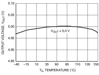
Figure 5. Output Voltage vs. Temperature 5.0 V Version
