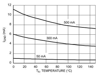
Figure 17. Ground Current vs. Temperature
