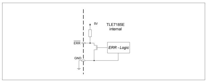
Figure 4 Structure of ERR output
