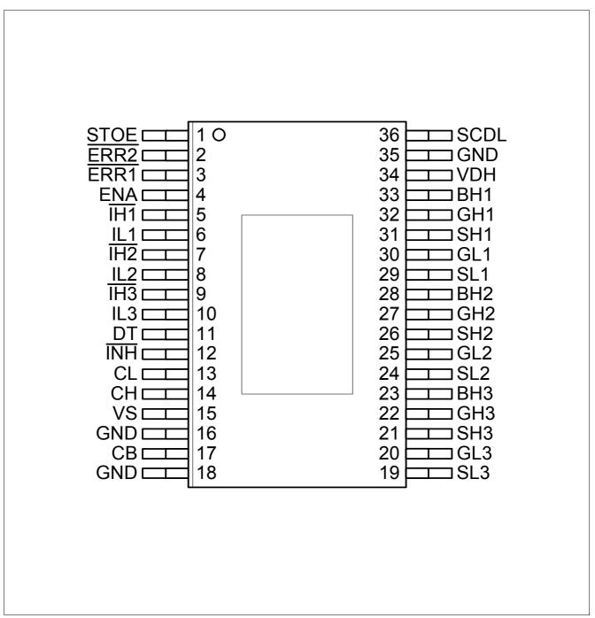
Figure 2 Pin Configuration
