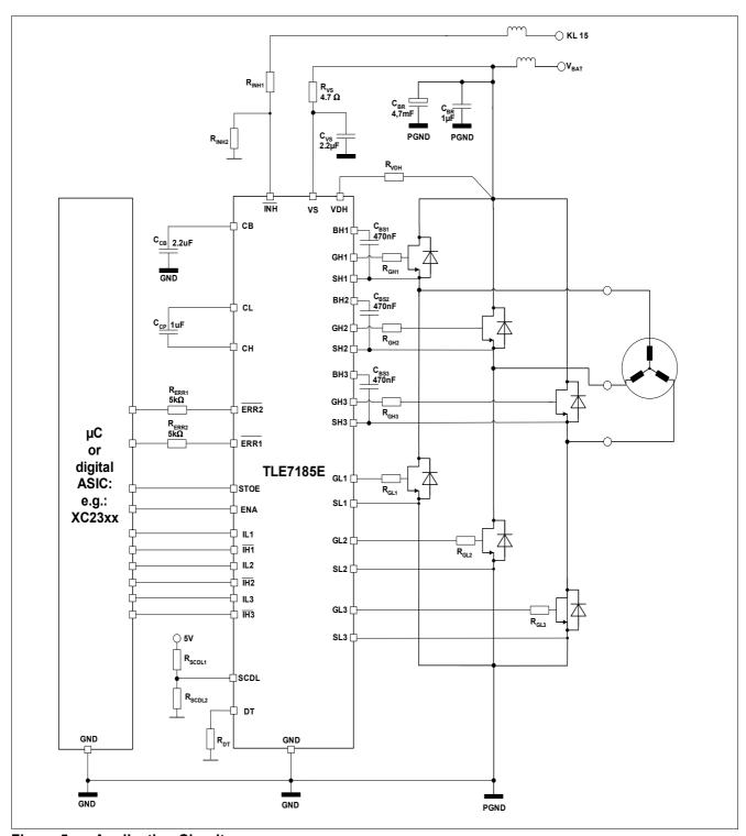
Figure 5 Application Circuit
