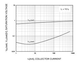
Figure 2. Collector-Emitter Saturation Voltage Base-Emitter Saturation Voltage
