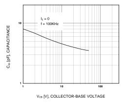
Figure 3. Collector-Base Capacitance
