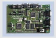
The EASY boards are including an Infineon 16 Bit-Microprocessor, the C165UTAH.
