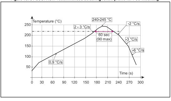
Figure 18: ST ECOPACK<sup>®</sup> recommended soldering reflow profile for PCB mounting
