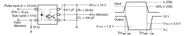
C∟ includes probe and stray wiring capacitance.
