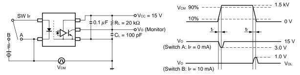
C∟ includes probe and stray wiring capacitance.
