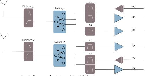
Block diagram of Inter-Band CA with dual-antenna
