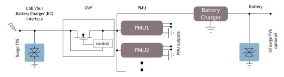
Mobile Device charging interface (Quick Charge, USB-PD)
