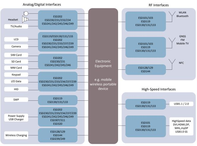
Interface protection with discrete ESD TVS diodes
