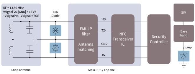
ESD protection for a differential NFC antenna system
