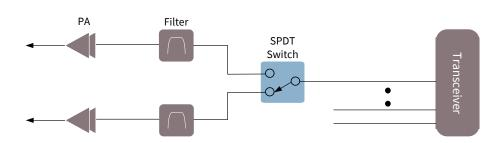
Application 1: band switching with CMOS SPDT switch
