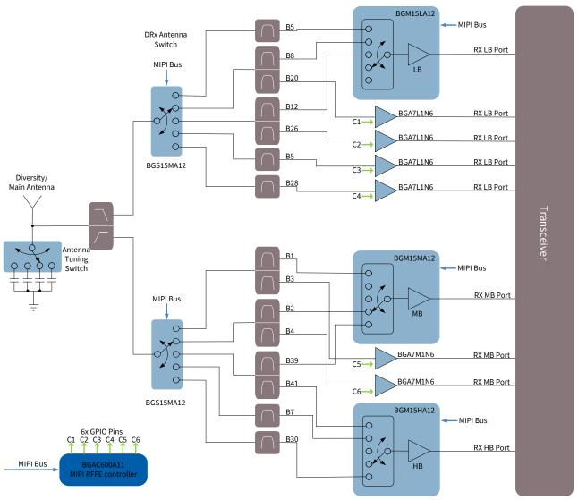
Single-antenna downlink RF FE Architecture for up to 5 CA
