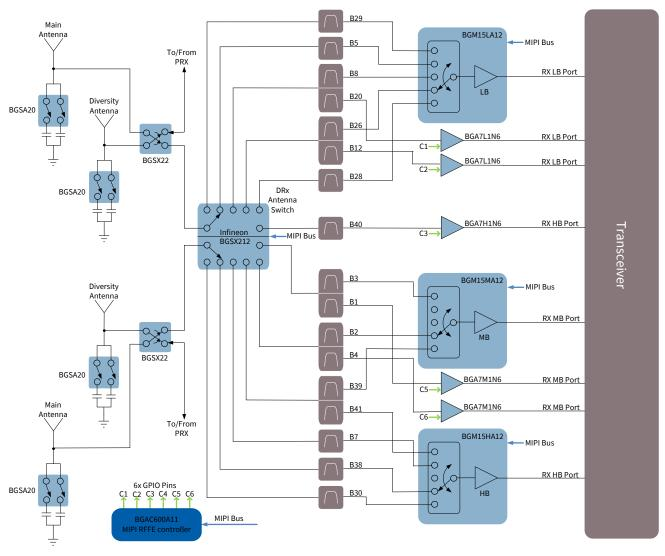
RF FE Architecture for Dual Antenna downlink up to 5 CA
