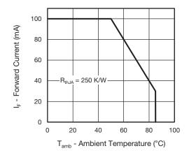
Fig. 1 - Power Dissipation Limit vs. Ambient Temperature
