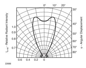
Fig. 6 - Relative Radiant Intensity vs. Angular Displacement
