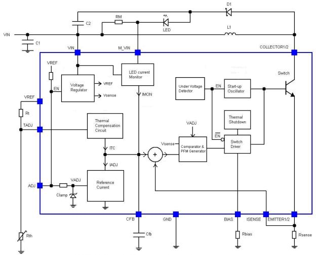
ZXLD1322 Block Diagram (showing external components)
