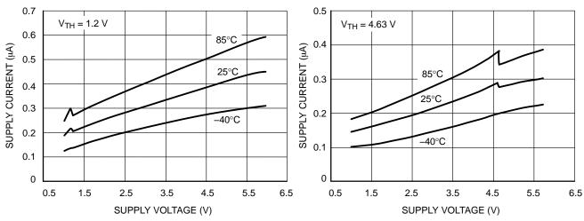
Figure 3. Supply Current vs. Supply Voltage
