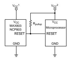
Figure 15. MAX803 RESET Output with Two Supplies
