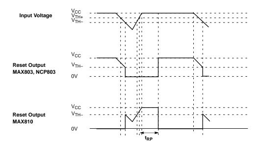
Figure 12. Timing Waveforms
