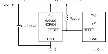
**Figure 1. Typical Application Diagram**
