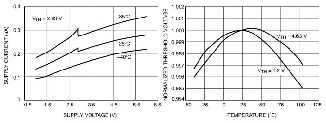
Figure 5. Supply Current vs. Supply Voltage
