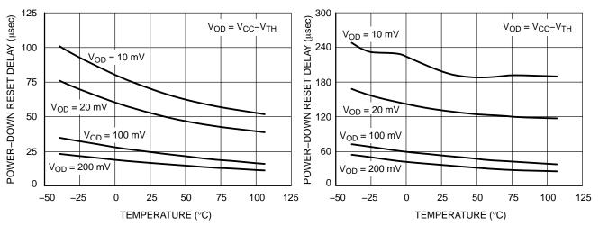
Figure 9. Power–Down Reset Delay vs. Temperature and Overdrive ( $V_{TH} = 1.2 V$ )
