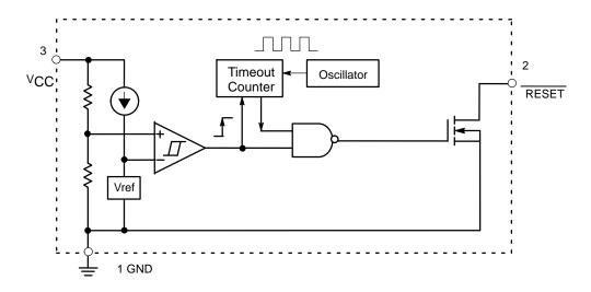
Figure 2. NCP803, MAX803 Series Open-Drain Active-Low Output
