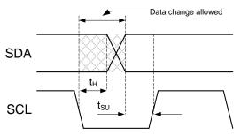
Figure 18. Data Transfer Timing
