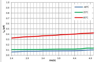
Figure 12. Quiescent Current vs. Input Voltage and Temperature, Auto Mode, Vout=1.15625 V
