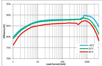
Figure 6. Efficiency vs. Load Current and Input Voltage,  $V_{\text{OUT}}$ =1.15625 V
