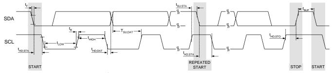
Figure 4. I<sup>2</sup>C Interface Timing for Fast Plus, Fast, and Slow Modes
