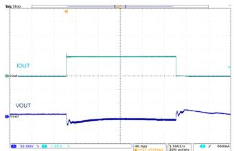
Figure 14. Line Transient, 3.6-4.2 V<sub>IN</sub>, 1.15625 V<sub>OUT</sub>, 10 μs Edge at 1 A Load
