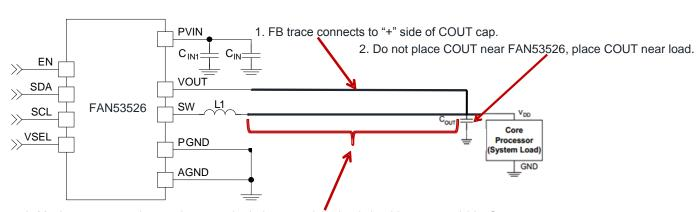
3. Maximum trace resistance between the inductor and the load should not exceed  $30m\Omega$ . For a 20mils wide PCB trace with 0.5mils thickness using 2oz. copper, a length of 0.5 inches gives a resistance of  $24.3m\Omega$ .
