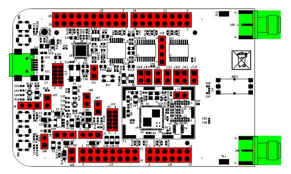
Figure 3. FRDM-KW019032 connector and header locations
