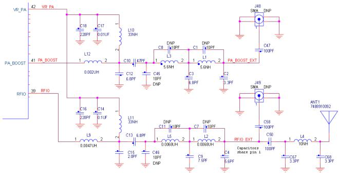
Figure 6. FRDM-KW019032 RF circuitry
