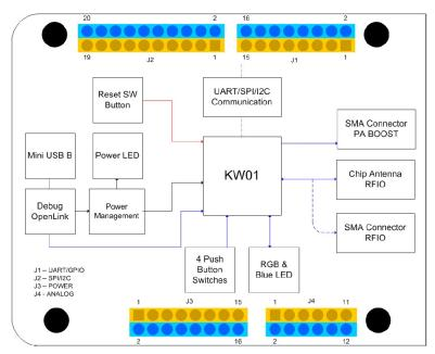
Figure 5. FRDM-KW019032 block diagram
