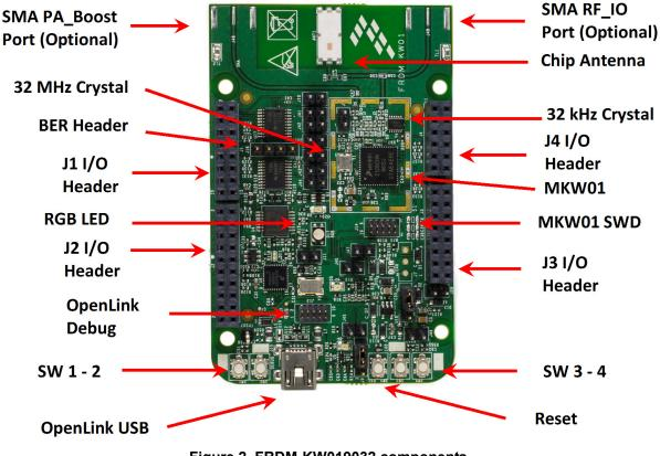
Figure 2. FRDM-KW019032 components
