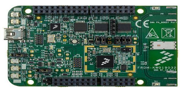
Figure 4. FRDM-KW019032 top side (component side) footprint
