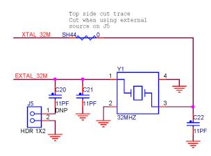
Figure 7. FRDM-KW019032 32 MHz reference oscillator circuit
