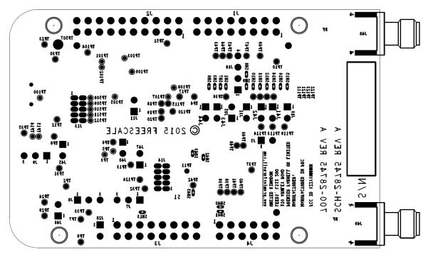
Figure 12. FRDM-KW019032 PCB test points
