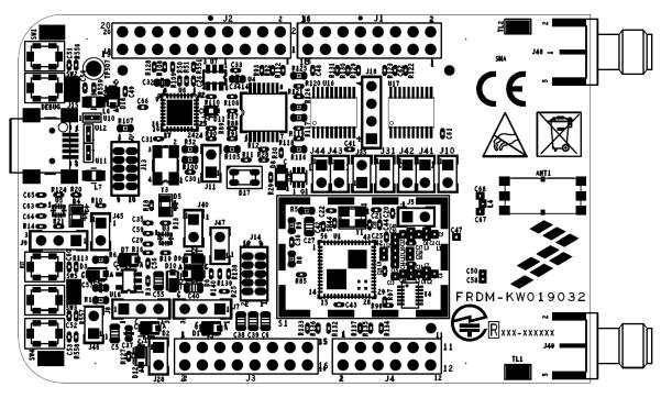
Figure 11. FRDM-KW019032 PCB component location (top view)
