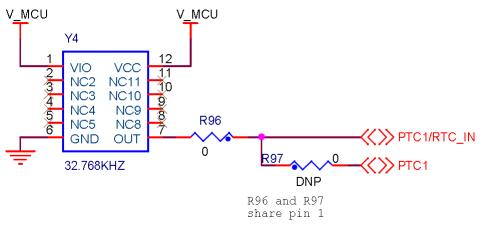
Figure 8. FRDM-KW019032 32.768 kHz optional oscillator circuit
