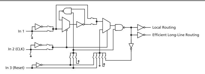
Figure 1-3 • Core Logic Tile
