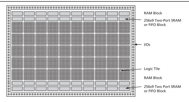
Figure 1-1 • The ProASICPLUS Device Architecture
