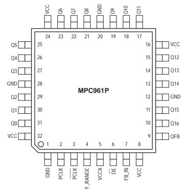
Figure 2. 32-Lead Pinout (Top View)
