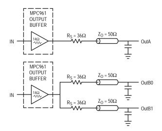
Figure 4. Single versus Dual Transmission Lines
