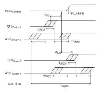
Figure 7. MPC961P max. device-to-device skew
