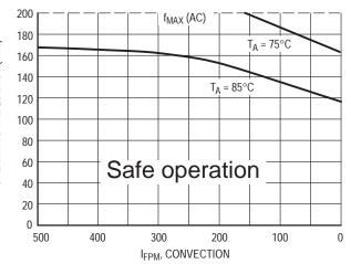
Figure 10. Maximum MPC961P frequency, V<sub>CC</sub> = 3.3V, MTBF 9.1 years, 4 pF load per line
