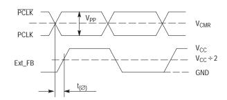
Figure 12. Propagation delay  $(t_{(O)})$ , static phase offset) test reference
