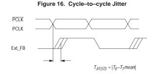
The deviation in  $t_0$  for a controlled edge with respect to a  $t_0$  mean in a random sample of cycles
