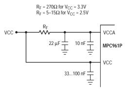
Figure 3. Power Supply Filter
