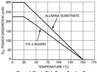
Figure 4. Steady State Power Derating Curve
