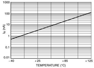
Figure 2. Typical Leakage Current versus Temperature
