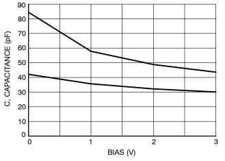
Figure 3. Typical Capacitance versus Bias Voltage (Upper curve is for unidirectional mode, lower curve is for bidirectional mode)
