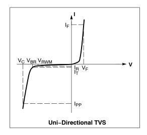
**ELECTRICAL CHARACTERISTICS** ( $T_A = 25^{\circ}C$  unless otherwise noted) **UNIDIRECTIONAL** (Circuit tied to Pins 1 and 3 or Pins 2 and 3)
