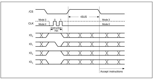
Figure 35b. Erase/Program Suspend Instruction (QPI Mode)
