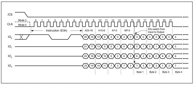
Figure 27a. Octal Word Read Quad I/O Instruction (Initial instruction or previous M5-4  $\neq$  10, SPI Mode only)
