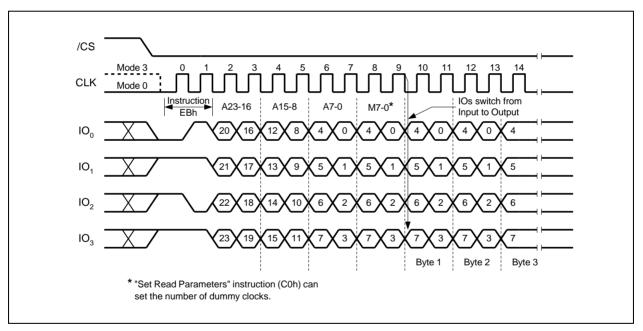
Figure 24c. Fast Read Quad I/O Instruction (Initial instruction or previous M5-4 $\neq$ 10, QPI Mode)
