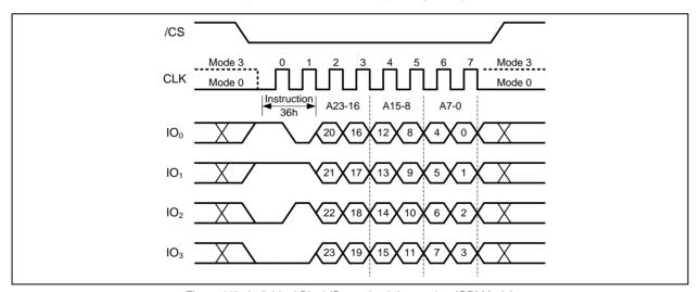
Figure 52b. Individual Block/Sector Lock Instruction (QPI Mode)
