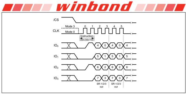
Figure 8b. Read Status Register Instruction (QPI Mode)
