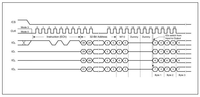
Figure 25a. Fast Read Quad I/O with 4-Byte Address Instruction (Initial instruction or previous M5-4≠10, SPI Mode only)
