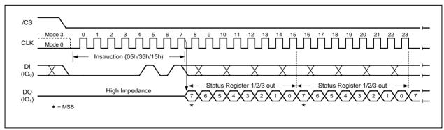
Figure 8a. Read Status Register Instruction (SPI Mode)
