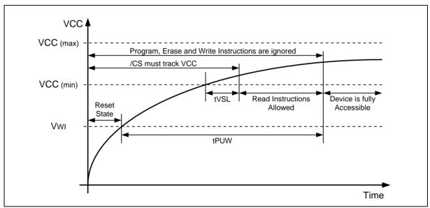
Figure 58. Power-up Timing and Voltage Levels
