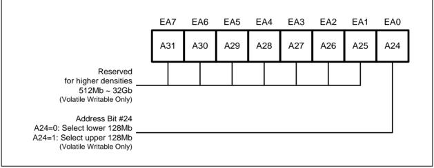
Figure 4e. Extended Address Register
