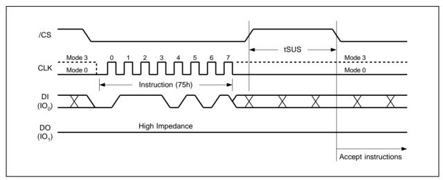
Figure 35a. Erase/Program Suspend Instruction (SPI Mode)
