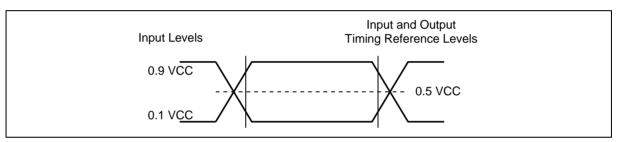
Figure 59. AC Measurement I/O Waveform
