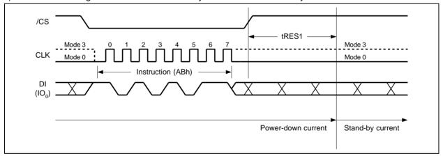
Figure 38a. Release Power-down Instruction (SPI Mode)
