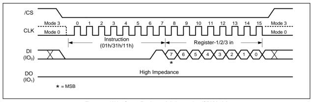
Figure 9a. Write Status Register-1/2/3 Instruction (SPI Mode)
