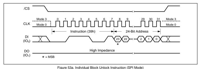
32-Bit Address is required when the device is operating in 4-Byte Address Mode
