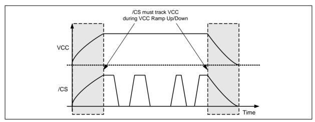
Figure 58b. Power-up, Power-Down Requirement
