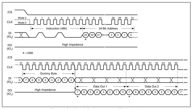
Figure 47. Read Security Registers Instruction (SPI Mode only) 32-Bit Address is required when the device is operating in 4-Byte Address Mode
