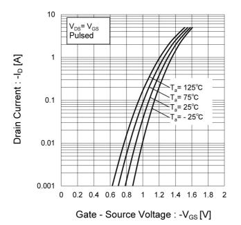
Fig.9 Gate Threshold Voltage vs.
