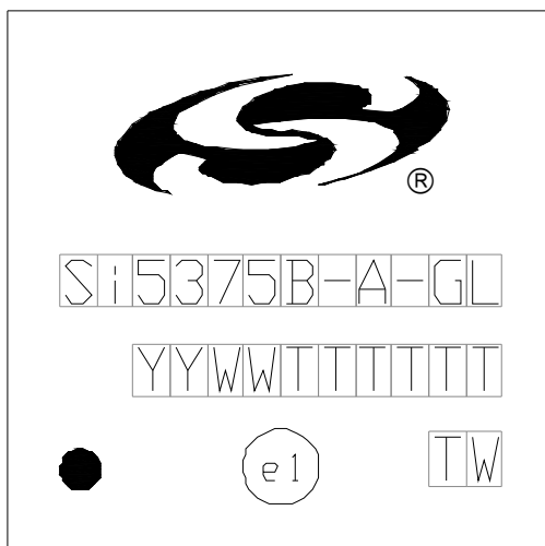
Figure 13. Si5375 Top Marking
