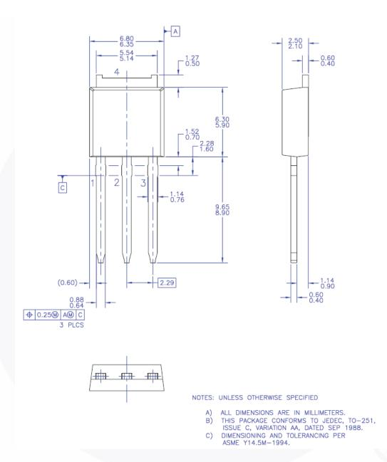
Figure 17. TO251 (I-PAK), Molded, 3-Lead
