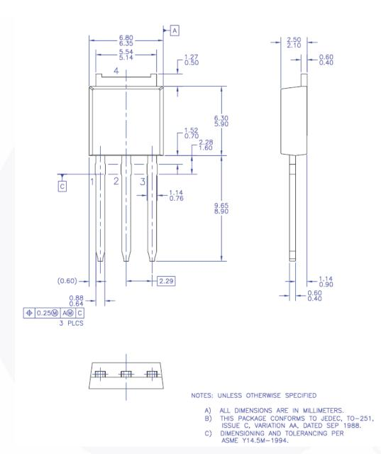
Figure 18. TO-251 (I-PAK), Molded, 3-Lead, Option AA
