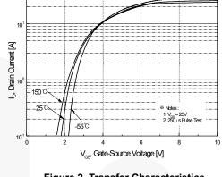
Figure 2. Transfer Characteristics
