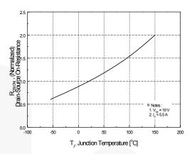
Figure 8. On-Resistance Variation vs. Temperature
