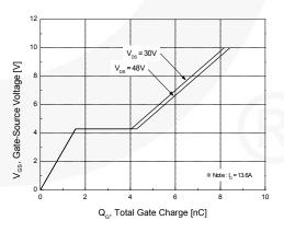
Figure 6. Gate Charge Characteristics
