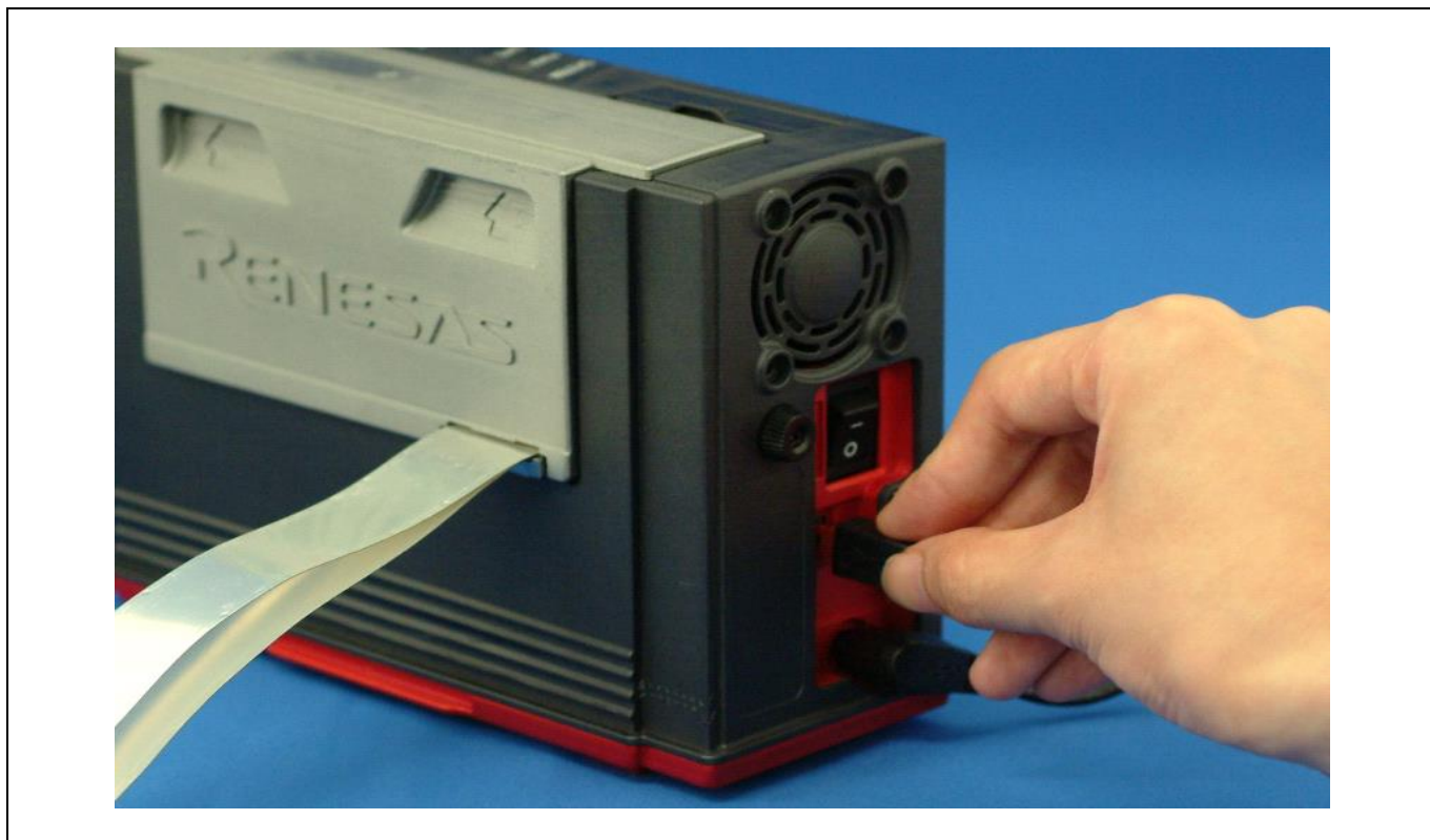
Figure 2.4 Connecting the host machine
