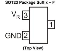
Pin 1 floating or connected to pin 2
