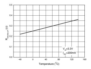
R<sub>DS(ON)\_LOW</sub> vs. Temperature
