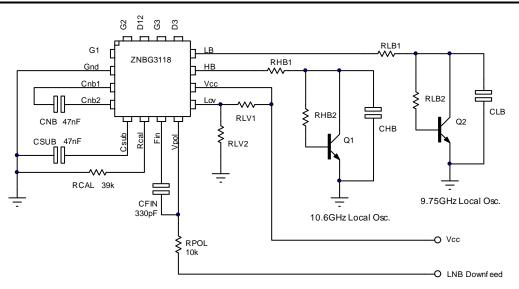
Figure 2 Applications circuit for the ZNBG3118 using Bi-polar oscillators
