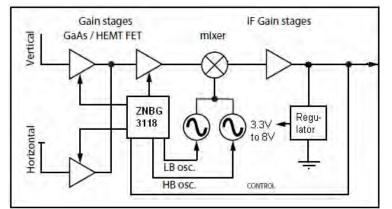
Figure 1 Typical single universal LNB system diagram
