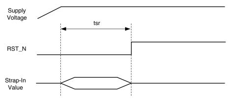
Figure 10. Reset Timing
