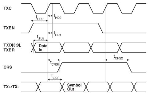
Figure 6. 100BASE-T MII Transmit Timing
