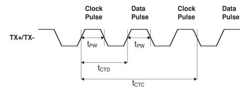
Figure 8. Auto-Negotiation/Fast Link Pulse Timing
