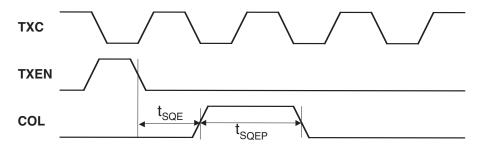
Figure 5. 10BASE-T MII Transmit Timing
