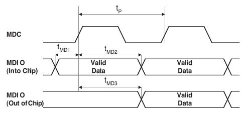
Figure 9. Serial Management Interface Timing
