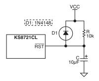
Figure 12. Recommended Circuit for Interfacing with CPU/FPGA Reset
