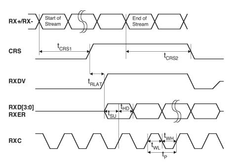
Figure 7. 100BASE-T MII Receive Timing
