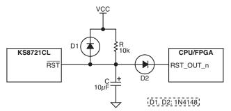
Figure 11. Recommended Reset Circuit.
