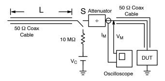
Figure 7. Simplified Schematic of a Typical TLP System
