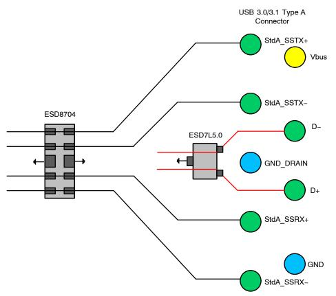
Figure 14. USB 3.0/3.1 Standard Layout Diagram
