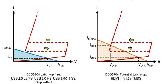
Figure 16. Example Load Lines for Latch-up Free Applications and Applications with the Potential for Latch-up
