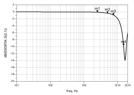
Figure 13. ESD8704 Insertion Loss
