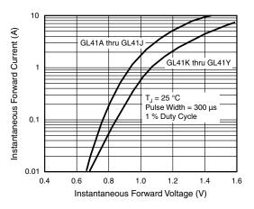
Fig. 3 - Typical Instantaneous Forward Characteristics
