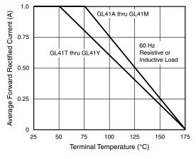
Fig. 1 - Forward Current Derating Curve
