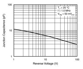
Fig. 5 - Typical Junction Capacitance
