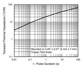
Fig. 6 - Typical Transient Thermal Impedance
