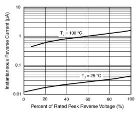
Fig. 4 - Typical Reverse Characteristics
