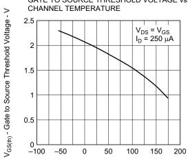
T<sub>ch</sub> - Channel Temperature - °C
