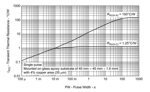
TRANSIENT THERMAL RESISTANCE vs. PULSE WIDTH (NP40N10YDF)
