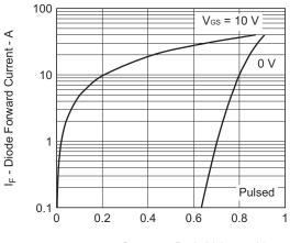
$V_{F(S-D)}$  - Source to Drain Voltage - V
