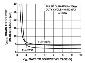
Figure 11. R<sub>DSON</sub> vs. Gate Voltage
