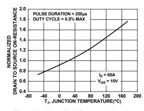
Figure 12. Normalized R<sub>DSON</sub> vs. Junction Temperature
