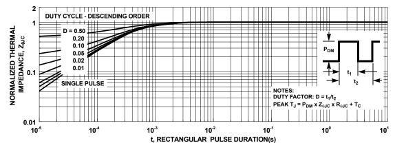
Figure 3. Normalized Maximum Transient Thermal Impedance
