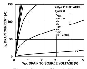
Figure 9. Saturation Characteristics
