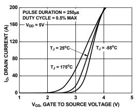
Figure 7. Transfer Characteristics
