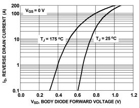
Figure 8. Forward Diode Characteristics
