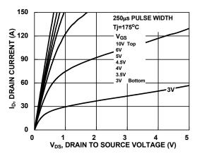
Figure 10. Saturation Characteristics
