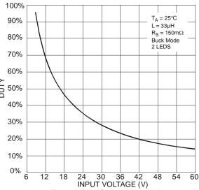
Figure 8 Duty Cycle vs. Input Voltage
