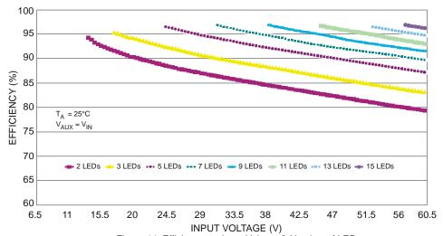
Figure 14 Efficiency vs. Input Voltage & Number of LED
