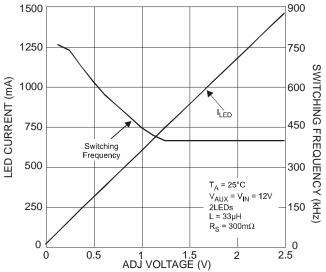
Figure 5 Buck LED Current, Switching Frequency vs. V<sub>ADJ</sub>
