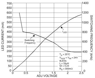
Figure 6 Buck-Boost LED Current, Switching Frequency vs. V<sub>ADJ</sub>
