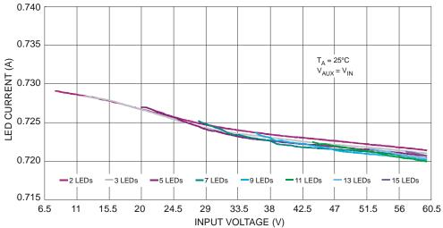
Figure 12  $I_{LED}$  vs. Input & Number of LED
