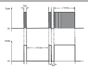
Figure 32 PWM Dimming Minimum and Maximum Pulse
