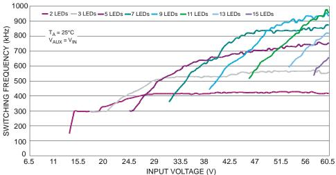
Figure 13 Frequency ZXLD1370 - Buck Mode - L47µH
