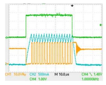
The PWM pin can be used to put the device into standby. Taking the PWM pin low (<0.4V) for more than 25ms (typically 15ms) the device will enter its standby state and most of the internal circuitry is switched off and residual quiescent current will be typically  $90\mu$ A. In particular, the STATUS pin will go down to GND while the FLAG and REF pins will stay at their nominal values.
