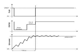
Figure 36 Diagnostic During Start-Up
