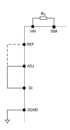
Figure 25 Setting LED Current in Buck Configuration
