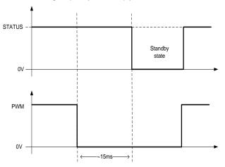
Figure 33 Standby State from PWM Signal
