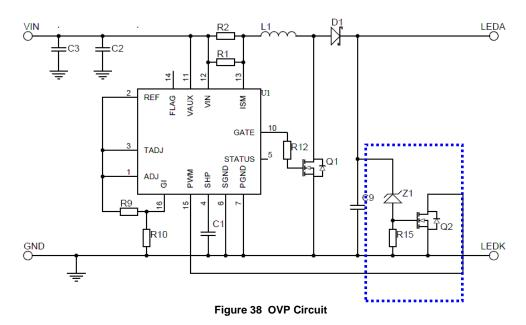
The zener voltage is determined according to:  $V_Z = V_{LEDMAX} + 10\%$  where  $V_{LEDMAX}$  is maximum LED chain voltage.
