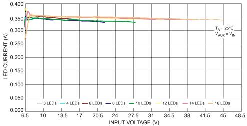
Figure 15 I<sub>LED</sub> vs. Input Voltage & Number of LED
