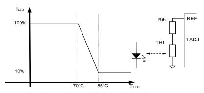
Thermal network response in Buck configuration with: Rth =  $1.8k\Omega$  and TH1= $10k\Omega$  (beta =3900)
