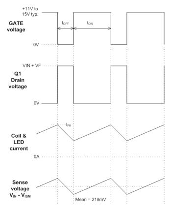
Figure 22 Operating Waveforms (Buck Mode)
