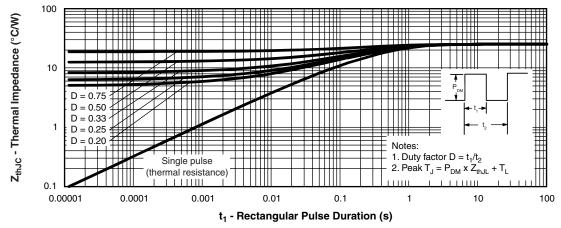
Fig. 4 - Maximum Thermal Impedance Z<sub>thJL</sub> Characteristics
