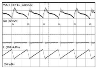
Figure 27. Steady-State Waveform for  $V_{\text{OUT}}$ , Switch Voltage, and Inductor Current for 7 LEDs
