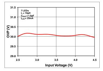
Figure 14. OVP vs. Input Voltage: FAN5346S20X
