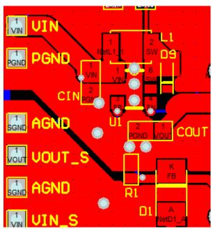
Figure 30. Reference PCB Layout
