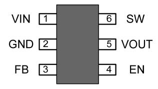
Figure 3. Pin Assignments, Top View
