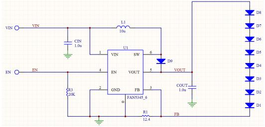
Figure 29. Reference Application Schematic Diagram
