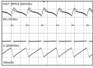
Figure 25. Steady-State Waveform for  $V_{\text{OUT}}$ , Switch Voltage, and Inductor Current for 6 LEDs
