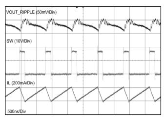
Figure 23. Steady-State Waveform for  $V_{\text{OUT}}$ , Switch Voltage, and Inductor Current for 5 LEDs
