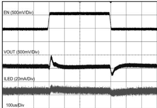
Figure 20. Line Transient Response for 6 LEDs
