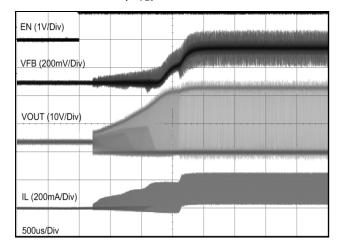
Figure 26. Startup Waveform for Switch Voltage, Inductor Current, V<sub>FB</sub>, and EN for 7 LEDs
