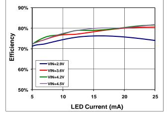
Figure 8. 7 LEDs: Efficiency vs. LED Current vs. Input Voltage
