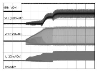
Figure 24. Startup Waveform for Switch Voltage, Inductor Current, V<sub>FB</sub>, and EN for 6 LEDs
