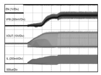
Figure 22. Startup Waveform for Switch Voltage, Inductor Current, V<sub>FB</sub>, and EN for 5 LEDs
