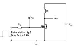
Switching time test circuit
