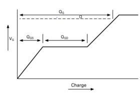
Basic gate charge waveform
