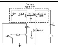
Gate charge test circuit
