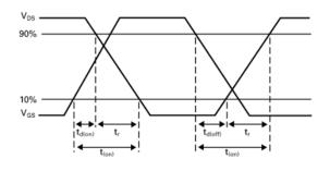
Switching time waveforms
