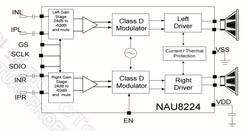
Figure 1: NAU8224Block Diagram
