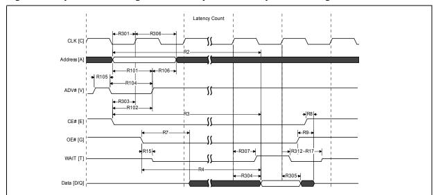
Figure 22: Synchronous Single-Word Array or Non-array Read Timing
