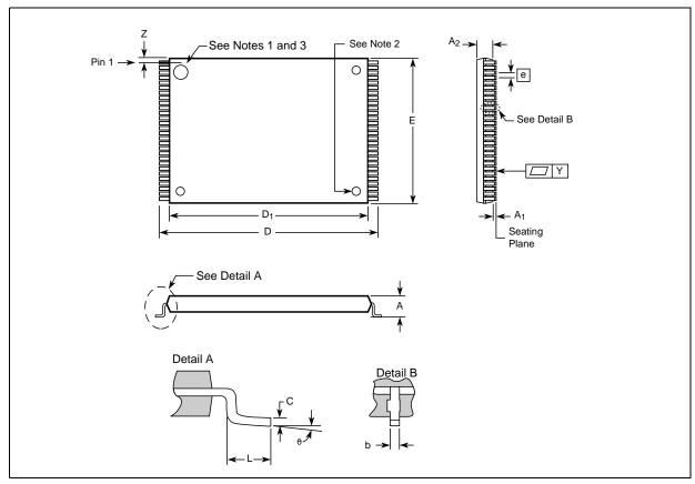
Table 1: TSOP Package Dimensions (Sheet 1 of 2)
