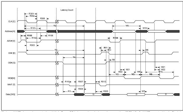
Figure 28: Synchronous Read-to-Write Timing
