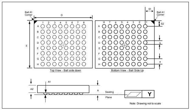
Easy BGA Package Dimensions for 10x13x1.2 mm (Sheet 1 of 2) Table 2:
