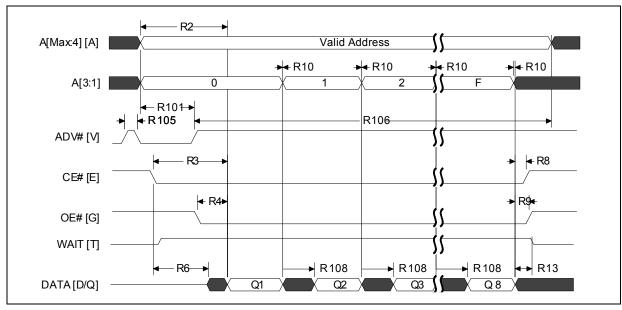
Figure 21: Asynchronous Page-Mode Read Timing
