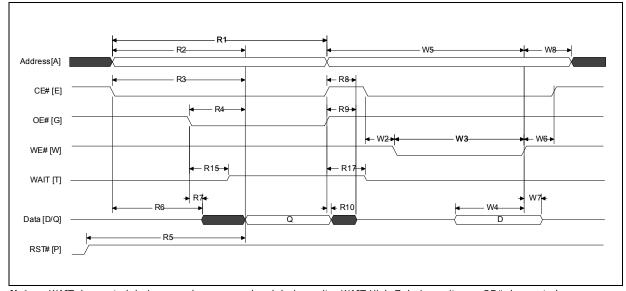
Figure 26: Asynchronous Read-to-Write Timing
