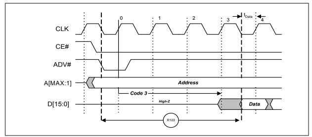
Figure 11: Example Latency Count Setting Using Code 3
