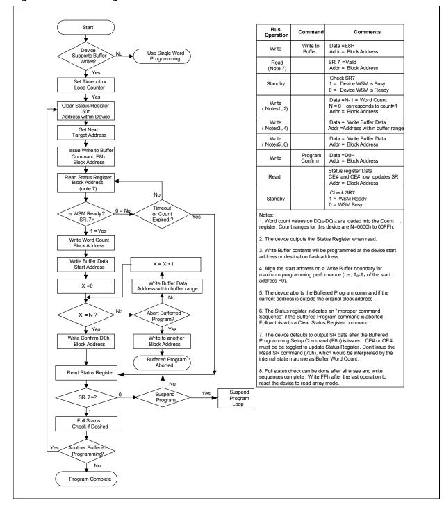
Figure 35: Buffer Program Flowchart
