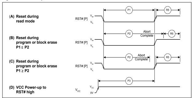
Figure 15: Reset Operation Waveforms
