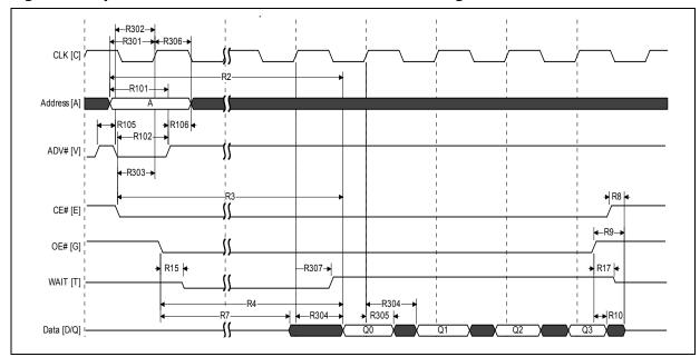
Figure 24: Synchronous Burst-Mode Four-Word Read Timing
