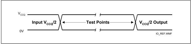
AC test inputs are driven at VCCQ for Logic "1" and 0 V for Logic "0." Input/output timing begins/ends at VCCQ/2. Input rise and fall times (10% to 90%) < 5ns. Worst case speed occurs at  $V_{CC} = VCCMin$ .
