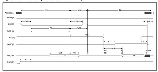
Figure 27: Write-to-Asynchronous Read Timing
