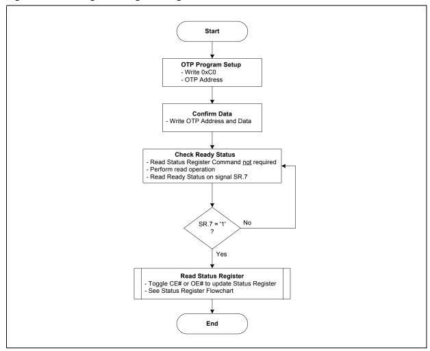
Figure 40: OTP Register Programming Flowchart
