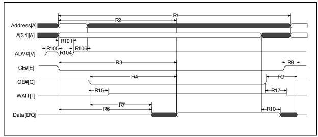
Figure 20: Asynchronous Single-Word Read (ADV# Latch)
