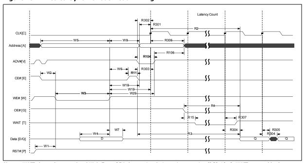
Figure 29: Write-to-Synchronous Read Timing
