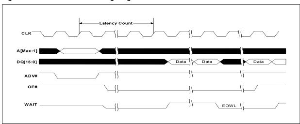
Figure 12: End of Wordline Timing Diagram
