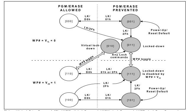
Figure 9: Block Locking State Diagram
