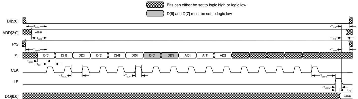
Figure 21. Latched-Parallel/Direct-Parallel Timing Diagram
