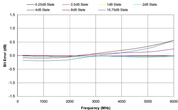
**Figure 6. 0.25 dB Attenuation Error vs. Frequency**
