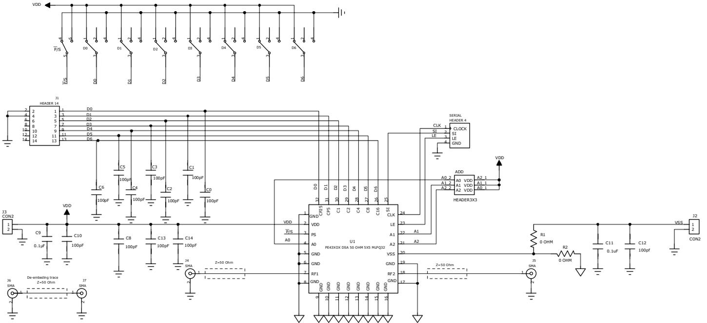
Note: Pin 26 is grounded. On the PE43601 pin 20 (shown as V<sub>SS</sub>) must also be grounded.
