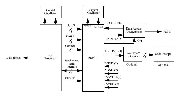
Figure 8. Modem Functional Interconnect Diagram
