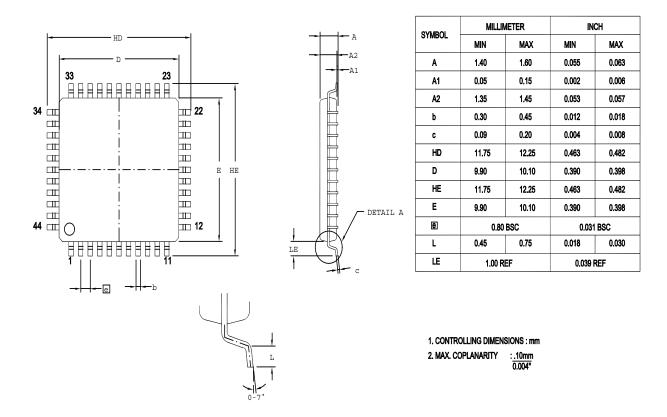
Figure 18. 44-Pin LQFP Package Diagram
