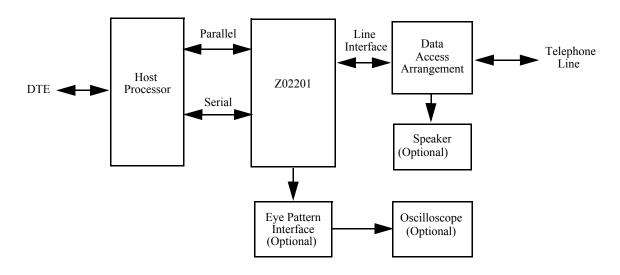
Figure 2. Z02201 System Block Diagram
