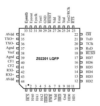
Figure 4. Z02201 44-Lead LQFP Pin Identification
