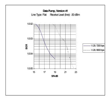
Figure 12. Bit Error Rate
