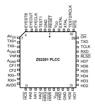
Figure 3. Z02201 44-Lead PLCC Pin Identification
