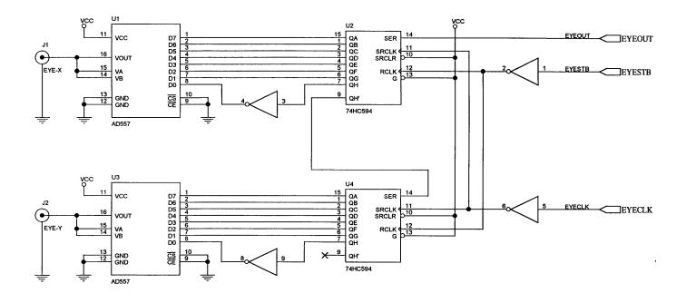
Figure 16. Eye Pattern Circuit
