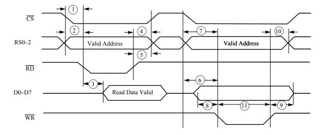
Figure 5. Microprocessor Interface Read/Write Diagram
