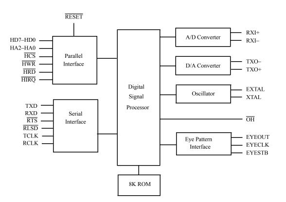
Figure 1. Z02201 Block Diagram
