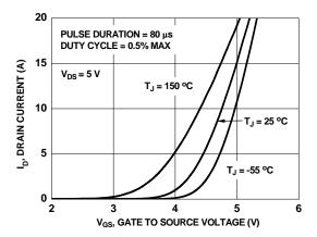
Figure 5. Transfer Characteristics
