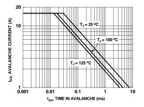
Figure 9. Unclamped Inductive Switching Capability
