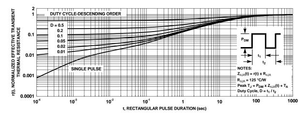
Figure 13. Junction-to-Ambient Transient Thermal Response Curve
