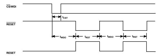
FIGURE 12. CS/WDI VS. RESET/RESET TIMING
