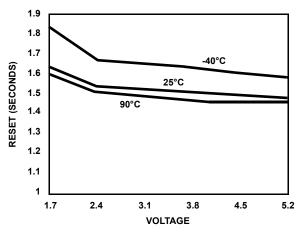
FIGURE 16. t<sub>WDO</sub> VS. VOLTAGE/TEMPERATURE (WD1, 0 = 1, 1)
