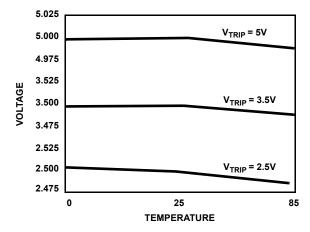
FIGURE 17. V<sub>TRIP</sub> vs. Temperature (programmed at 25°C)
