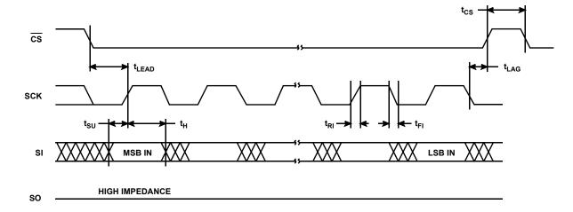
FIGURE 11. SERIAL INPUT TIMING
