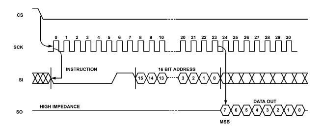
FIGURE 5. READ EEPROM ARRAY SEQUENCE
