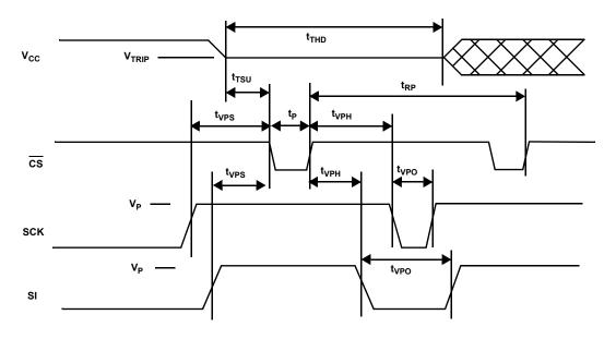
FIGURE 13.  $V_{TRIP}$  SET CONDITIONS
