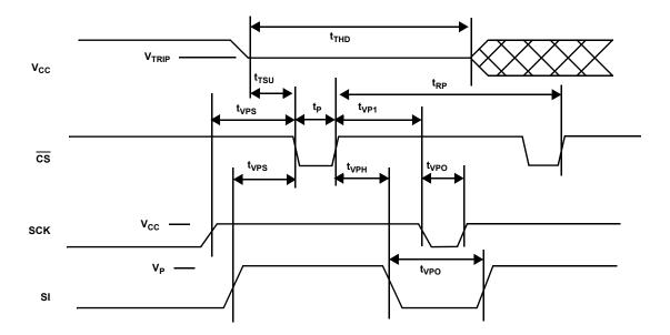
FIGURE 14.  $V_{TRIP}$  RESET CONDITIONS
