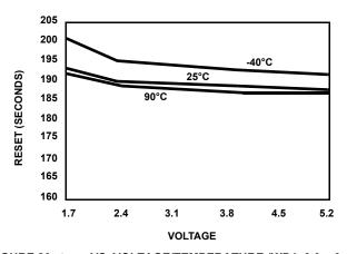
FIGURE 20.  $t_{WDO}$  VS. VOLTAGE/TEMPERATURE (WD1, 0 0 = 0, 1)
