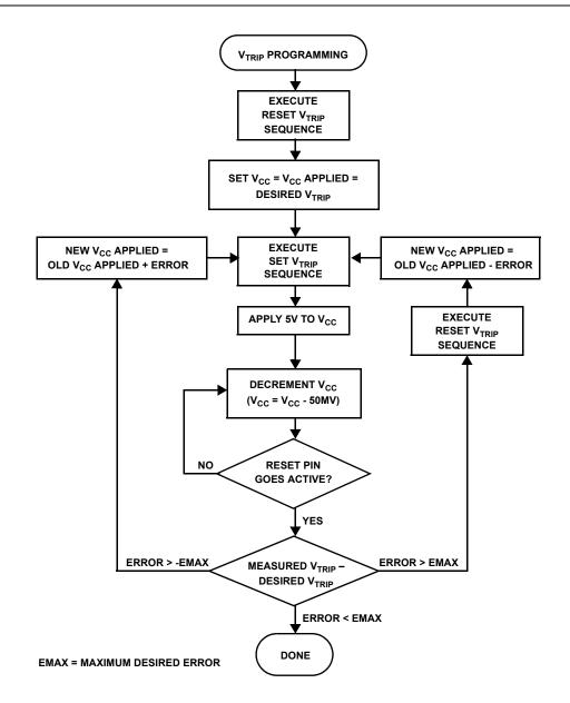
FIGURE 3.  $V_{TRIP}$  PROGRAMMING SEQUENCE FLOW CHART
