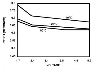
FIGURE 18. t<sub>WDO</sub> VS. VOLTAGE/TEMPERATURE (WD1, 0 = 1, 0)
