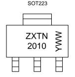
ZXTN 2010 = Product Type Marking Code YWW = Date Code Marking Y or  $\overline{Y}$  = Last Digit of Year (ex: 5= 2015) WW or  $\overline{W}W$  = Week Code (01~53)
