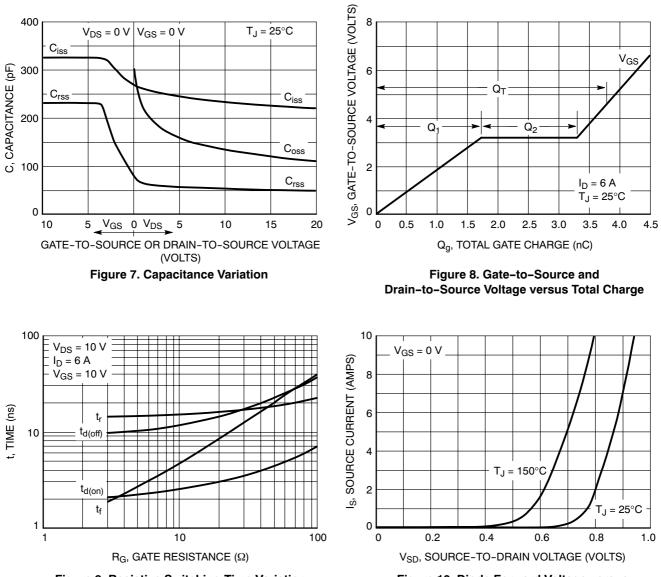
Figure 9. Resistive Switching Time Variation versus Gate Resistance
