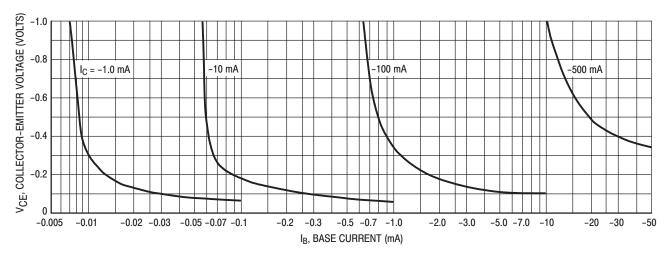
Figure 4. Collector Saturation Region
