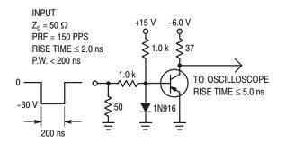
Figure 2. Storage and Fall Time Test Circuit
