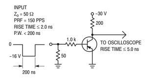
Figure 1. Delay and Rise Time Test Circuit
